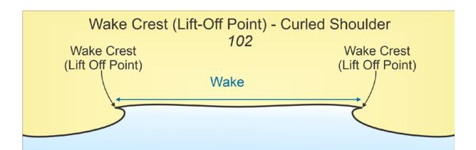
The wave curl is the point of the wave crest (lift-off point).
