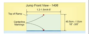
(B) Surface. The surface of the ramp out of the water shall be 210cm ±4.2cm long, with the waterline marked by the center of a transverse line of contrasting color of a width equal to the total 8.4cm. The width of the ramp surface shall be a minimum of 1.20m and a maximum of 1.50m with parallel sides. The surface of the jump ramp shall be flat with a maximum deviation of ±1cm from a plane. The overall length of the ramp surface shall be a minimum of 3.6m.
